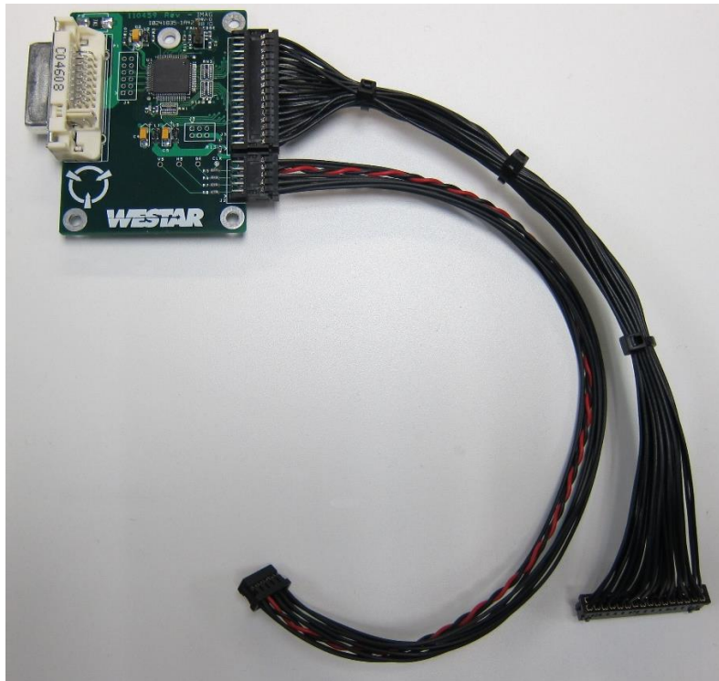
Figure 1: 110459, shown with separately available cabling to connect to a Westar VPx board.
