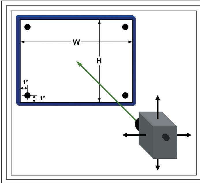
**Fig. 3:** TCO '05 Notebooks standard, paragraph B.2.3.2, "Luminance Uniformity Measurement," requires the LMD to be positioned in four corner positions perpendicular to the screen surface.
