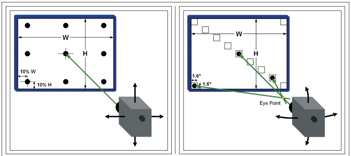
**Fig. 1:** VESA FPDM standard, section 306-1, “Sampled Uniformity & Color of White Measurement,” requires the LMD to be positioned in five (or optionally nine) positions perpendicular to the screen surface.
