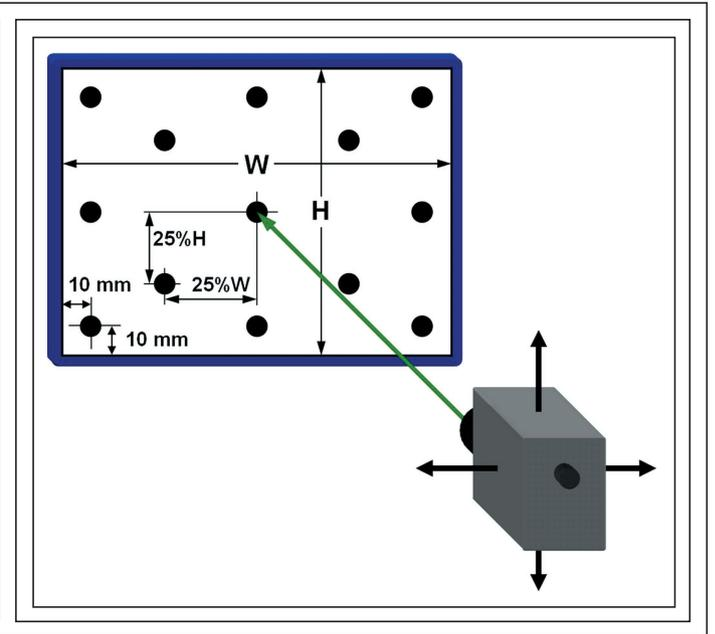
**Fig. 4:** SPWG standard, section 6.4, "White Uniformity Measurement," requires that the LMD be positioned in 13 positions perpendicular to the screen surface.
